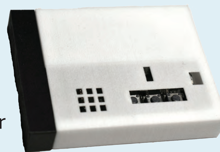
The SenseBee hardware in its 3D printed enclosure
