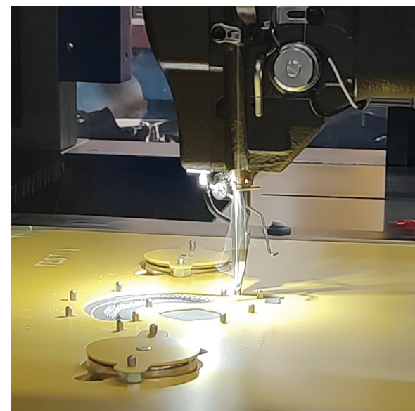
The machine stitches the fabric together along set paths
