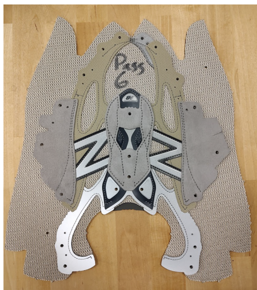
990v6 Shoe Top Assembly created in the stitching process
