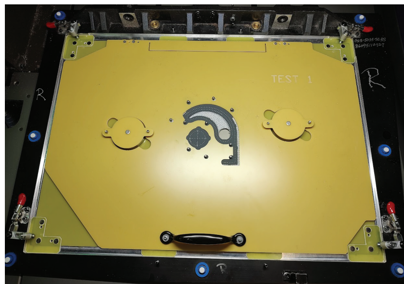
Pallets used to accurately load fabric into the stitching machines
